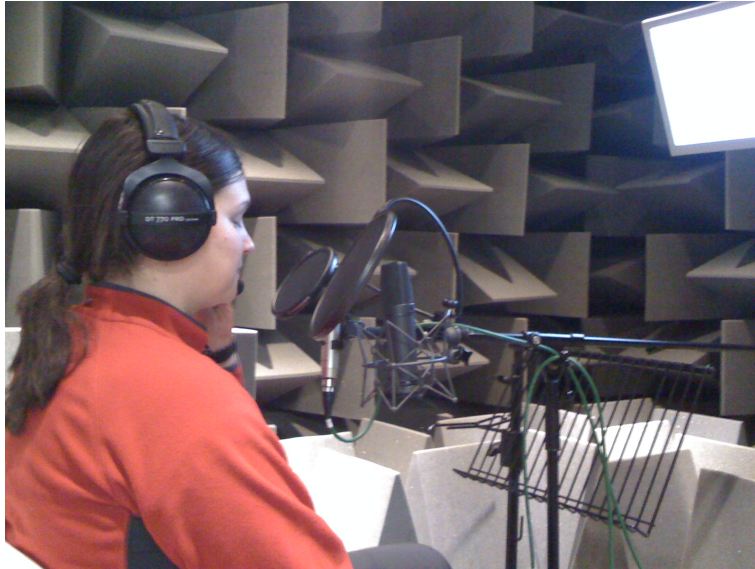
Figure 3.1: Studio setup for recordings. Left microphone is a Sennheiser MKH 800 and the right one is a Neumann u89i. The headset has a DPA 4035 microphone mounted on it.
